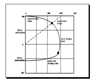
Figure 3-1 Generator MVAr versus MW Capability
