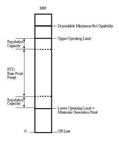
Figure 4-2 Generating Unit Operating Characteristics
