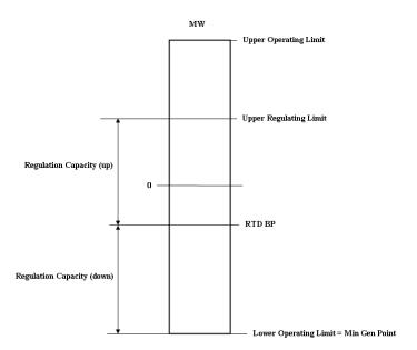
Figure 4-4 LESR with RTD Managing Energy Level; Equal Reg Up and Reg Down
