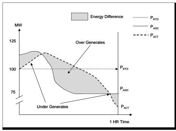
Figure 4-7 Error in Performance (30-Second Bandwidth not Included)
